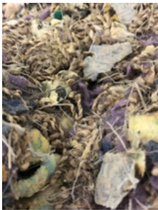
Shredding using a 40 mm screen
