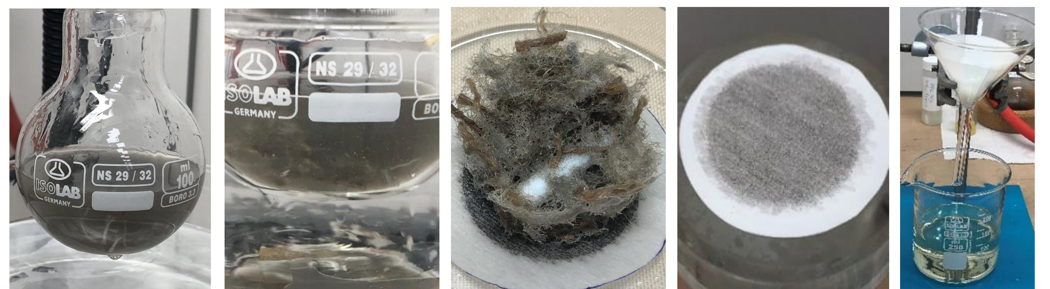
Figure 3: Undissolved non-PP components and pigments were removed by successive filtration steps.
