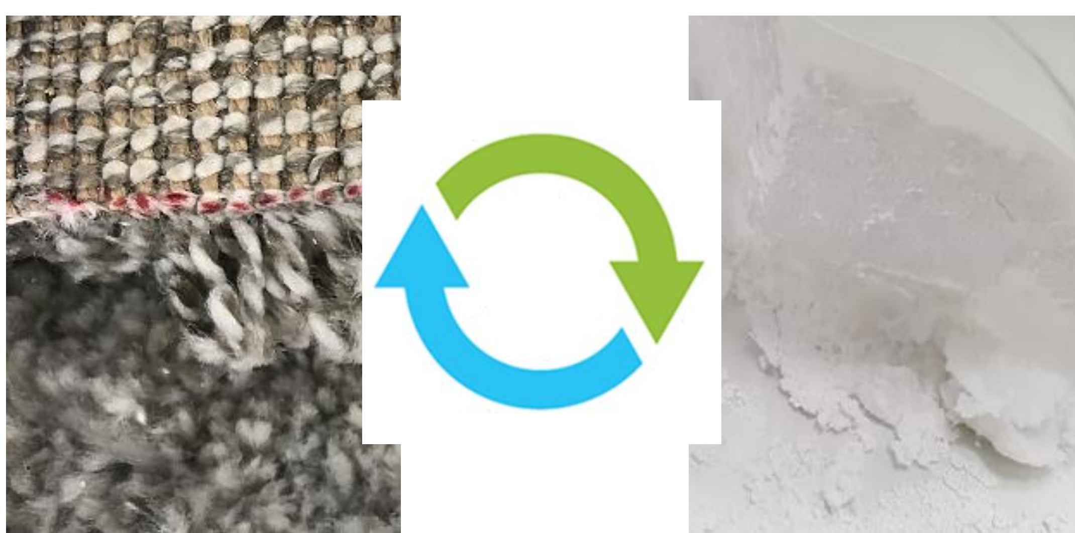
Figure 4: Photographs of the waste carpet and PP obtained from the waste carpet by the recycling process.
